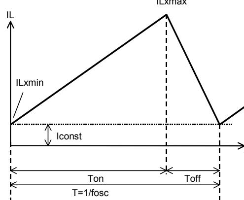
There are two modes, or discontinuous mode and continuous mode for the PWM step-up switching regulator depending on the continuous characteristic of inductor current.
